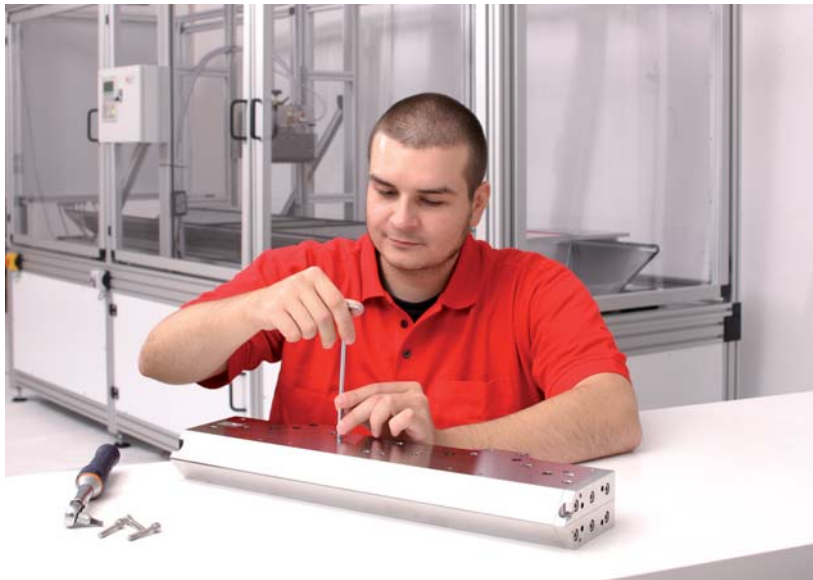
Assembly of a 500 mm wide FMP precision die
