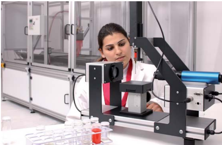
Measurement of the surface tension and contact angle in the FMP TECHNOLOGY GMBH laboratory
