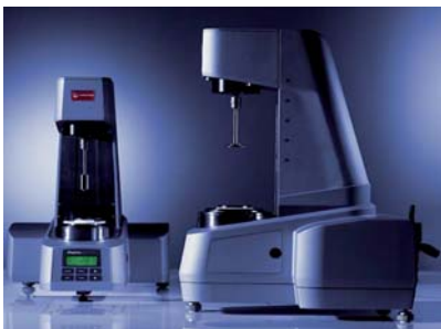
Measurement device for the analysis of the fluid viscosity depending on the shear rate
