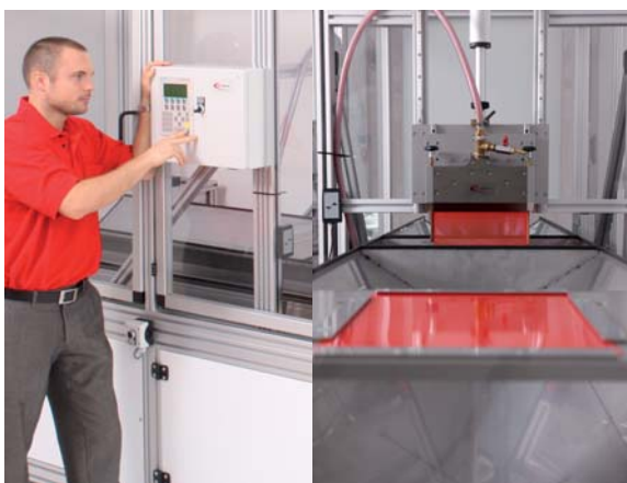
Coating of substrates on a laboratory scale machine
